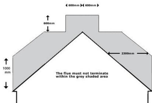
1. The point of outlet of a chimney must be a minimum of 600mm above the highest point of contact of the chimney and the roof, if the centre of the flue is within 600mm of the highest point / ridge,
